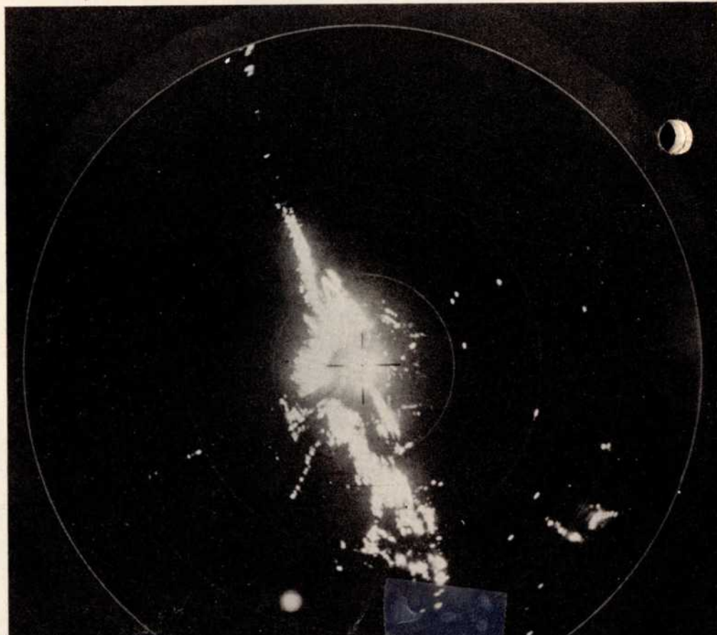
MEW PPI on 200-mi. range, low beam. Presumable surface target at 110°, 150 miles. Large indication at 125°, 150 miles checks in range, bearing and shape with Grand Bahama Island. Series of indications at 340°, 190 miles does not check with any logical target, but is on the coast line, near Jacksonville.
