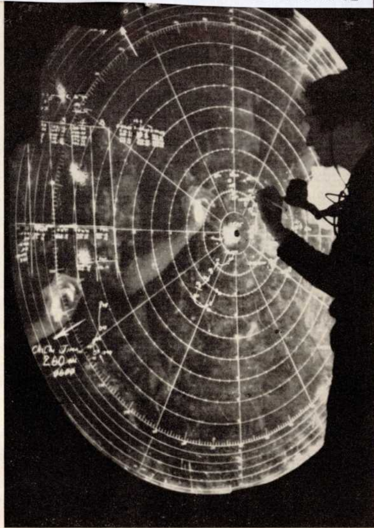
Giant eye. On this edge-lit lucite plot in an Essex class carrier CIC was displayed the air picture as told by reports from own and other ships' radar.
