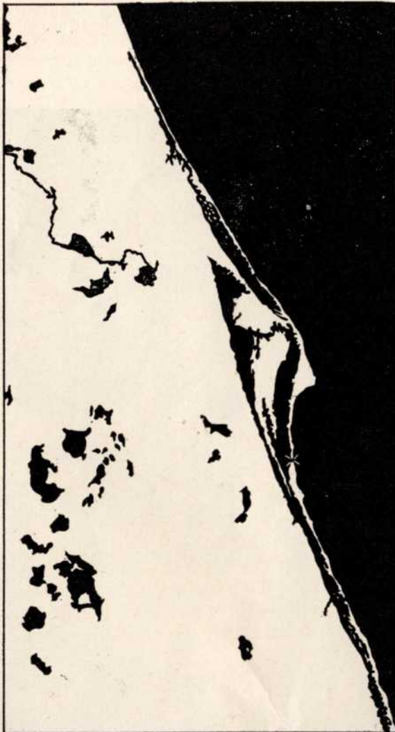
MEW PPI scope, 90-mi. range, low beam antenna. Exceptional mapping of Banana River, Indian River and associated land masses (compared with chart). Surface targets in NE quadrant from 62 to 82 miles, others inside 50-mi. range marker. A night interception exercise at 125°, 40 miles has been completed and fighter is seen breaking away in a port turn during exposure time (1½ minutes for all photos).
