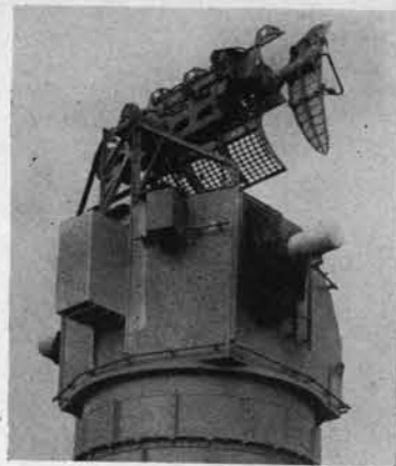
The Mark 22 (small antenna to the right) installed alongside the Mark 4 radar. Gun director is Mark 37 with round-backed shield.
