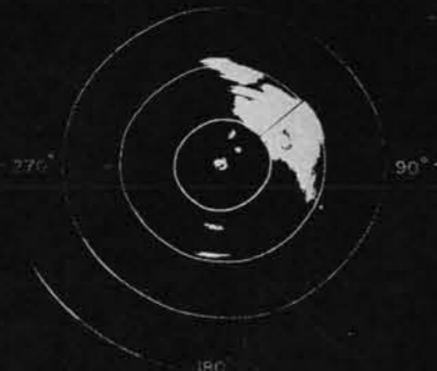
Actual PPI photo of Oahu made at mast height from the exact position simulated above.
