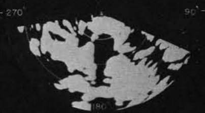
Simulated PPI photo of Smoky Mountains, made in test that proved validity of RPD.
