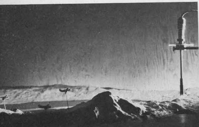
Permanent Echo would conceal the first plane (left), shadow the second, but the third would be spotted by the radar.
